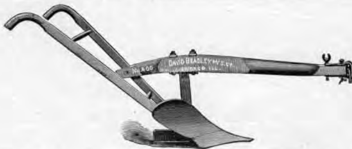
STEEL CORN PLOW—Wood Beam, Slip Share. Hardened Moldboard. Single Shin, Low Landside, Slip Share.
