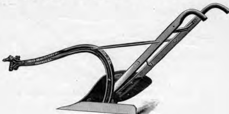
STEEL STUBBLE PLOW—Steel Beam, Long-Bar Share. Hardened Moldboard. Low Landside.
