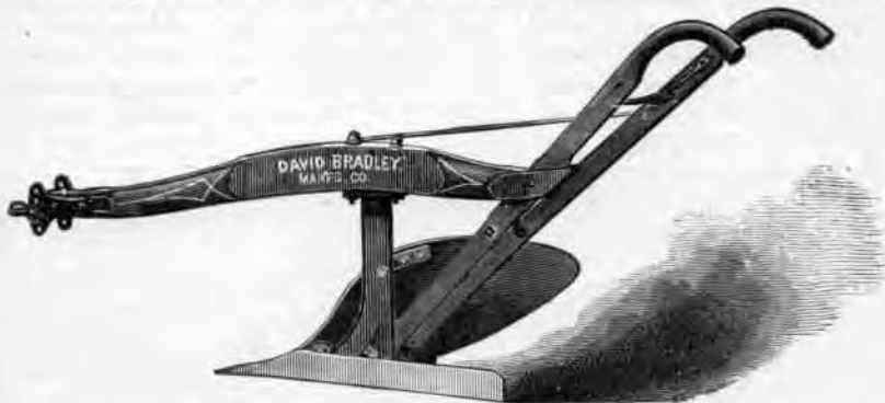
STEEL STUBBLE PLOW—Wood Beam, Long Bar Share. Hardened Moldboard. Low Landside.
