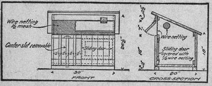
Plan of the Model Coop, Built of Tongue and Groove Material. Entire Top Can Be Lifted Off Bottom.
