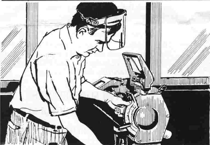
Are you ready to use the emory wheel or milling or cutting machine? Before putting it in motion, turn the grinding wheel around by hand to make certain it is not cracked or chipped and that it is dressed square. Adjust work rest, spark deflector and the illuminated deflector shield.
