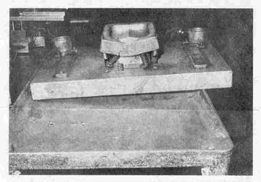
Pictured is a die that was broken recently through the carelessness of an employee. As a result the cost of repairing it was approximately \$300.00. Even worse, the die was out of commission for three days at a time when it was badly needed. It may even have resulted in some employees being sent home for lack of parts in Assembly.
